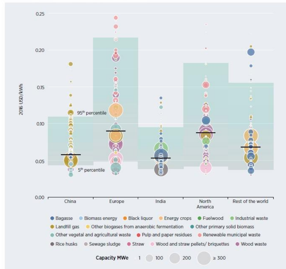
Figure 7.4 Levelised cost of electricity by project and weighted averages of bioenergy-fired electricity generation by feedstock and country/region, 2000-2016
